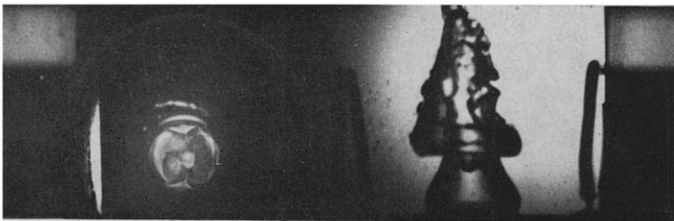
FIG. 8. Bubble with zero waiting time and irregular microlayer . Test liquid ethanol; gross heat flux 69.8 \text{ kW/m}^2 , pressure 25.4 \text{ kN/m}^2 subcooling 4.8^\circ\text{C} .
